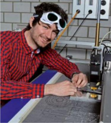
Textiles are "limp". Their form is unstable and they can form creases involuntarily. They are thin and can quickly become overheated by the laser and the textile will be damaged. Different "Textile surfaces", as the expert calls them, also behave differently during processing. Because of their stitches knitted and crocheted fabrics are trickier candidates than "smooth" fabrics.
